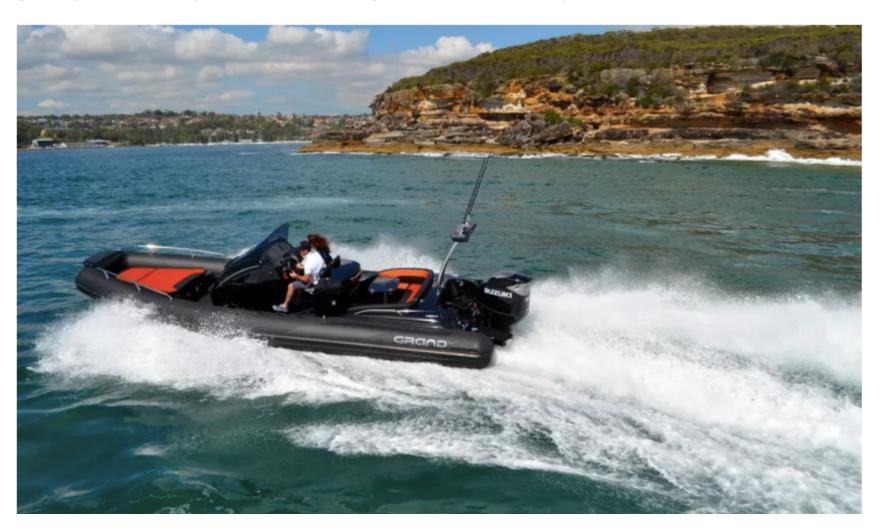
The deep-vee fibreglass hull is designed for a smooth ride, while the heavy-duty hypalon tubes, with overpressure valve, create incredible stability at rest and underway. The boat features a self-bailing cockpit, so no issues if you take some green water when crossing the bar or beach.
