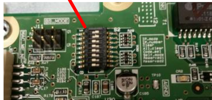
DIP Switches – 1 and 2 ON
