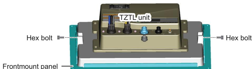
2. Place the NavNet TZtouch2 unit face-down on a soft, clean surface.
