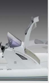
The front lifted seat allows the easy access to huge compartment into steering console.
