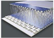
Double-wall drop stitch materials for high-pressure inflatable floors
