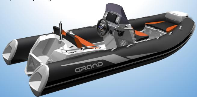
Safety handrails are fitted as standard on the port and starboard side of the ergonomically designed pilot/passenger seats and steering console. Stainless steel bow rails are also available as an option.
